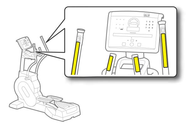
**Sensors**: levers and fixed handles have sensors for monitoring the heat rate (hand sensor), in the 700 and 700 SP versions of the equipment.
