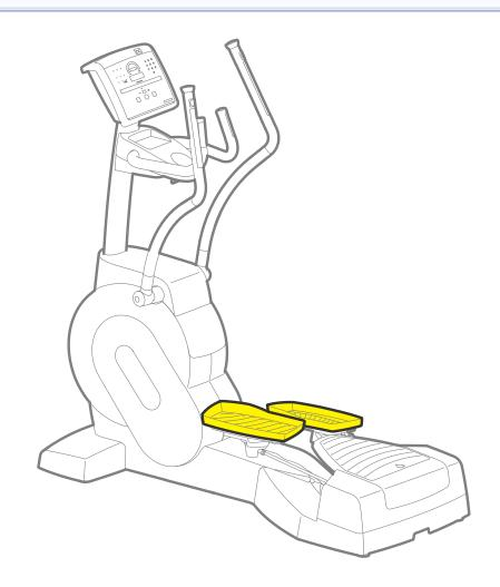
Pedals: the special configuration of the pedals permit the ankles to work under optimum conditions.
