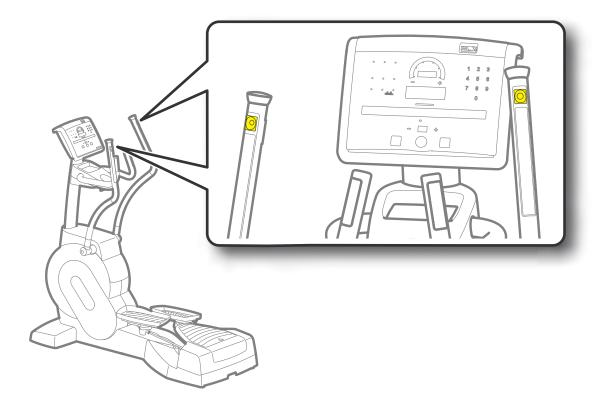
Levers: these can be grasped by the user to perform the exercise with arm movements. The 700 and 700 SP versions have sensors for monitoring the heat rate (hand sensor) and the Fast Track Control to change the effort level.
