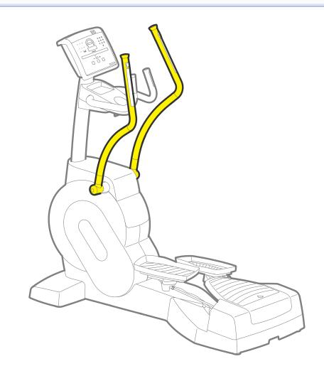
Levers: these can be grasped by the user to perform the exercise with arm movements. The 700 and 700 SP versions have sensors for monitoring the heart rate (hand sensor) and the Fast Track Control to change the effort level.
